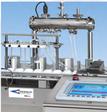
Cozzoli Peristaltic Pump with 316L Stainless Steel Supply Manifold
